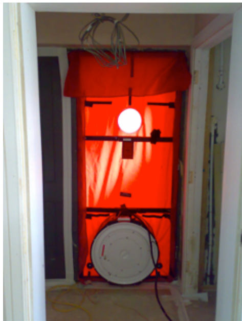
Fig 11: An airtightness blower door test in progress. In this case in the UK
