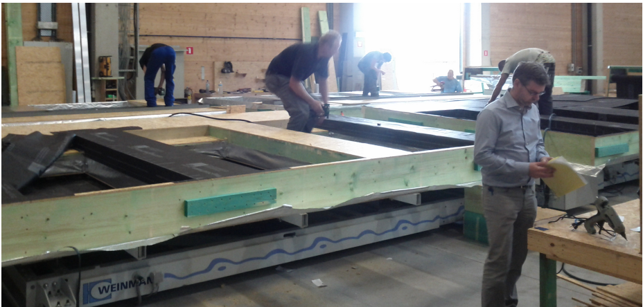
FIG. 4: PREFAB PANEL PRODUCTION LINE
